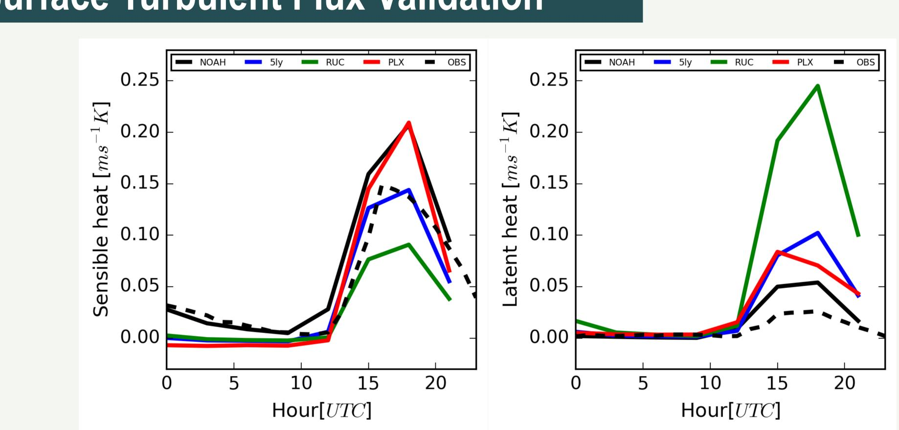
Figure 8. Surface and latent heat flux validation for urban areas: Model simulated fluxes are compared to turbulent flux measurements at a representative urban site using a Campbell CSAT3 sonic anemometer and a Campbell KH20 higrometer
