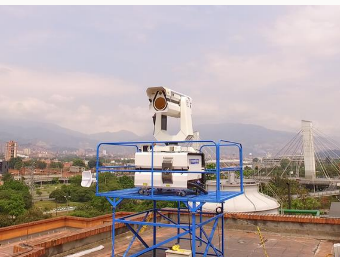
Fig 3. Depolarization Lidar located at the bottom of the valley
